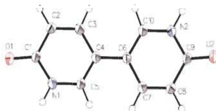
Fig. S6 Thermal atomic displacement ellipsoid plot of 1a crystallized at 80 °C in EtOH/DMF. The ellipsoids of non-hydrogen atoms are drawn at 50% probability level, hydrogen atoms are represented by a sphere of arbitrary size.
