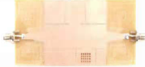
Fig. 3. Fabricated SIW-based multiresonator (N=2) for temperature and humidity detection.
