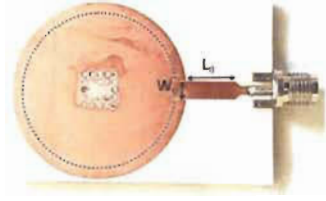
Fig. 5 Fabricated SICCR-based humidity sensor
