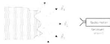
Fig3 Principle of receiving EM signal by a radiometer sensor
