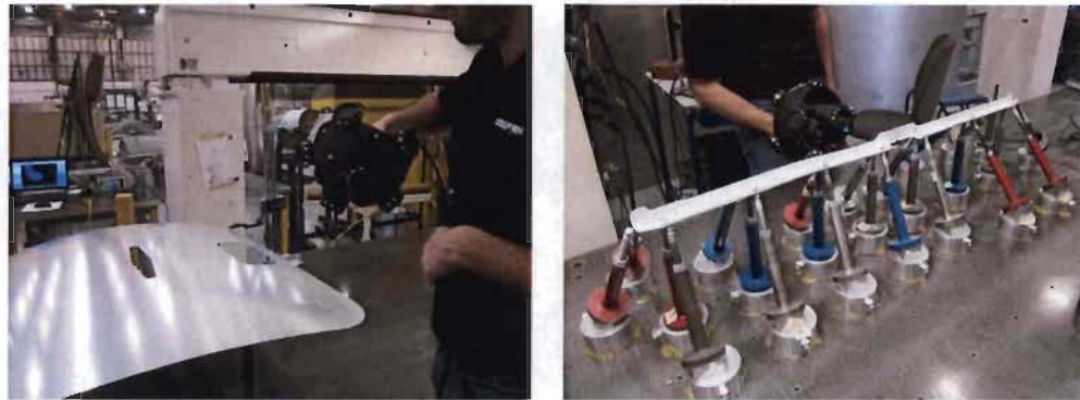
Figure 4-2: Surface data acquisition by a handy scanner.
