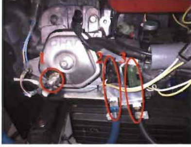
Fig. 2. The modified bi-fuel generator: 1-camshaft sensor; 2-hydrogen injector and 3-Gasoline injector
