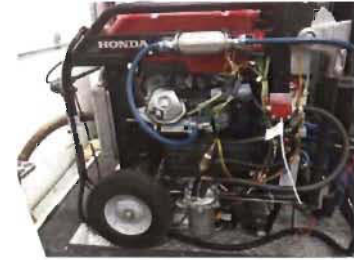
Fig. 2: Test bench of a generator bi-fuel
