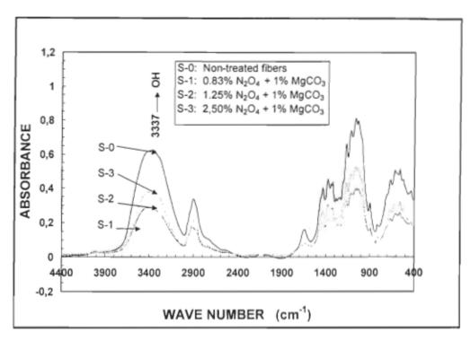
FIGURE 4.30 FTIR absorbance peaks of oxidised bleached kraft softwood fibres at oxidation rates of 0, 0.83, 1.25 and 2.50% N<sub>2</sub>O<sub>4</sub>/fiber + 1% MgCO<sub>3</sub>.
