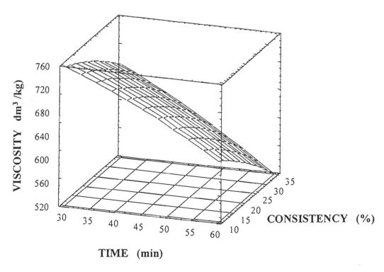
FIGURE 4.16 The estimated surface response of viscosity as a function of pulp consistency and oxidation time.
