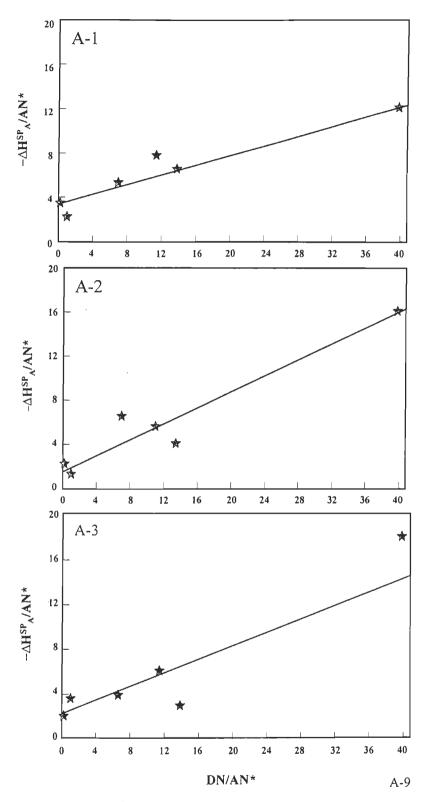
FIGURE A.12 Plot of - $\Delta H^{SP}_A/AN^*$  versus DN/AN\* for the oxidised aspen bleached kraft fibres at N<sub>2</sub>O<sub>4</sub>/fibre of 0.83% (A-1), 1.25% (A-2) and 1.66% (A-3).
