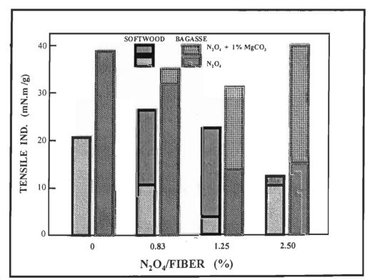
FIGURE 4.92 The effect of the addition 1.0 % MgCO<sub>3</sub> on tensile index during oxidation by  $N_2O_4$ .
