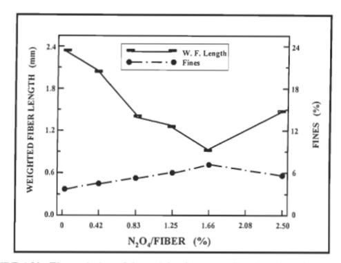
FIGURE 4.80 The variation of the weighted average fibre length and percentage of fines of the oxidised bleached kraft softwood as a function of percentage of N<sub>2</sub>O<sub>4</sub>/fiber.
