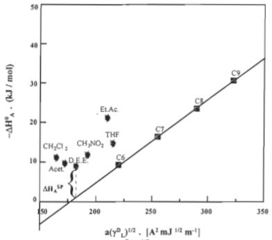
FIGURE 4.62 Plot of  $-\Delta H_A$  versus a  $(\gamma^D_L)^{1/2}$  of the alkane and polar probes of the untreated bleached kraft aspen fibres.
