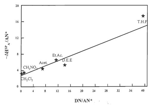
FIGURE 4.67 Plot of  $-\Delta H^{SP}_A/AN^*$  versus DN/AN\* for the oxidised bleached kraft bagasse fibres with 2.5 % N<sub>2</sub>O<sub>4</sub> allowing the determination of the acceptor constant,  $K_A$  and donor constant,  $K_B$ .
