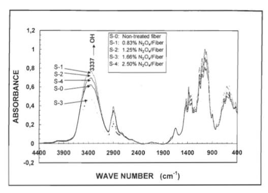
FIGUE 4.24 FTIR absorbance peaks of oxidised bleached kraft softwood fibres at different oxidation rates of 0, 0.83, 1.25, 1.66 and 2.50% N<sub>2</sub>O<sub>4</sub> /fiber.
