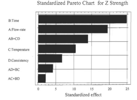
FIGURE 4.10 Standardised Pareto chart for the z strength of oxidised fibres of bleached kraft softwood.
