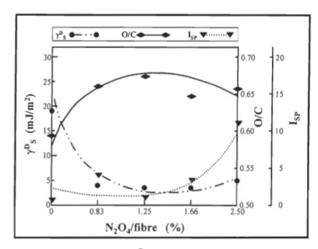
FIGURE 4.70 The relation between  $\gamma^D_S$  with the O/C ratio and the  $I_{SP}$  as the function of the percentage of  $N_2O_4$ /fibre for the softwood oxidised fibres.
