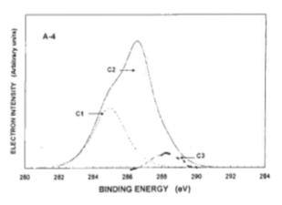
FIGURE 4.36 C(1s) peaks obtained from ESCA spectra of aspen oxidised by by  $N_2O_4$  at oxidation rates of 0 .0% (A-0), 0.83% (A-1), 1.25% (A-2), 1.66% (A-3) and 2.50% (A-4).
