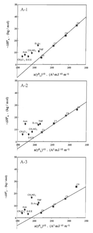
FIGURE A.9 Plot of  $-\Delta H_A$  versus  $a(\gamma^D_L)^{1/2}$  of the alkane and polar probes of the oxidised aspen bleached kraft fibres at N<sub>2</sub>O<sub>4</sub>/fibre of 0.83% (A-1) ,1.25% (A-2) and 1.66% (A-3).
