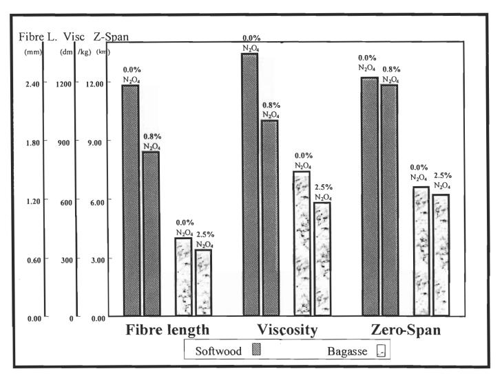
FIGURE 4.100 Factors affecting fibre strength of softwood and bagasse fibre oxidised by N<sub>2</sub>O<sub>4</sub> in presence of 1% MgCO<sub>3</sub>.
