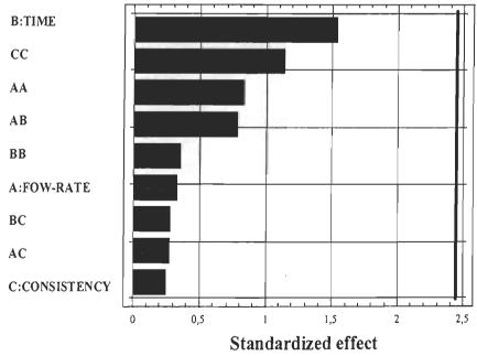
FIGURE 4.19 The standardised Pareto chart of brightness for the oxidation factors.
