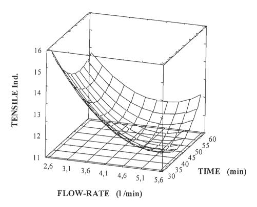
FIGURE 4.18 The estimated surface response of tensile index as a function of gas flow-rate and oxidation time.
