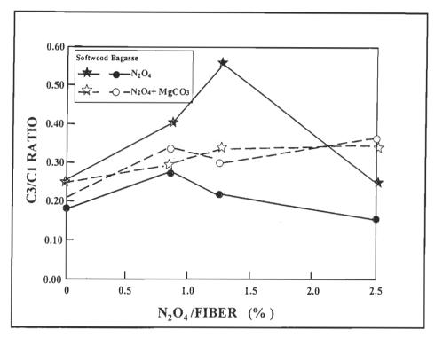
FIGURE 4.44 Plot of C3/C1 ratio of bleached kraft fibres of softwood and bagasse, versus the  $N_2O_4$  oxidation rate, in presence of 1% MgCO<sub>3</sub>.
