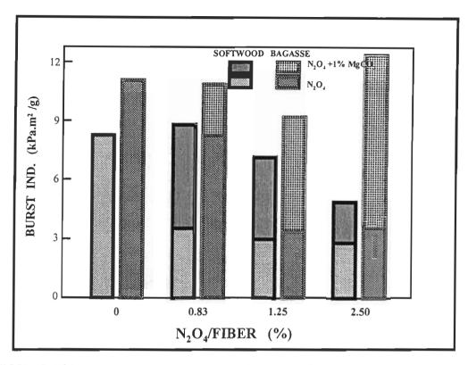
FIGURE 4.93 The effect of the addition 1.0 % MgCO<sub>3</sub> on burst index during oxidation by N<sub>2</sub>O.
