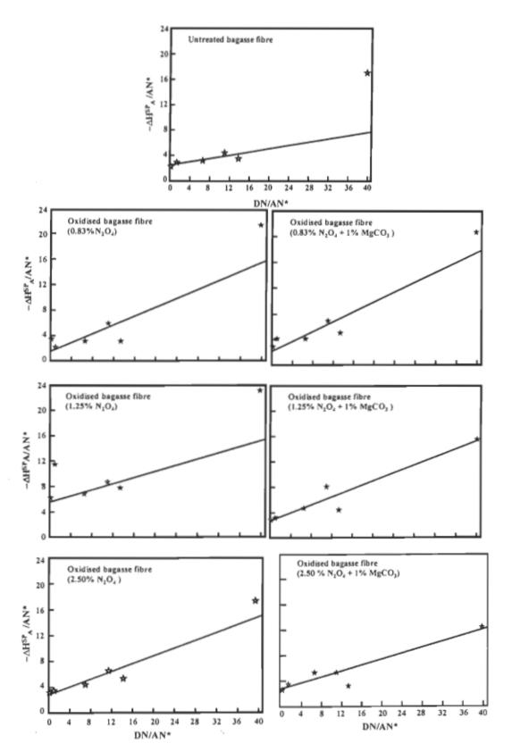
FIGURE 4.76 Plot of ΔH<sup>SP</sup><sub>A</sub>/AN\* versus DN/AN\* for untreated and oxidised bagasse fibres without MgCO<sub>3</sub> (left-side) and in presence of MgCO<sub>3</sub> (right-side).
