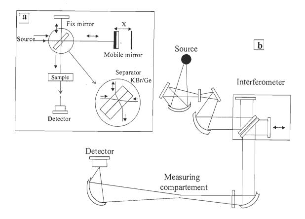
FIGURE 3.3 Optical assembling of Fourier transformer. a) 90° Michelson Interferometer. b) Optical diagram of spectrometer with single beam of Fourier transformer IFS 25 (Bruker association) (79).
