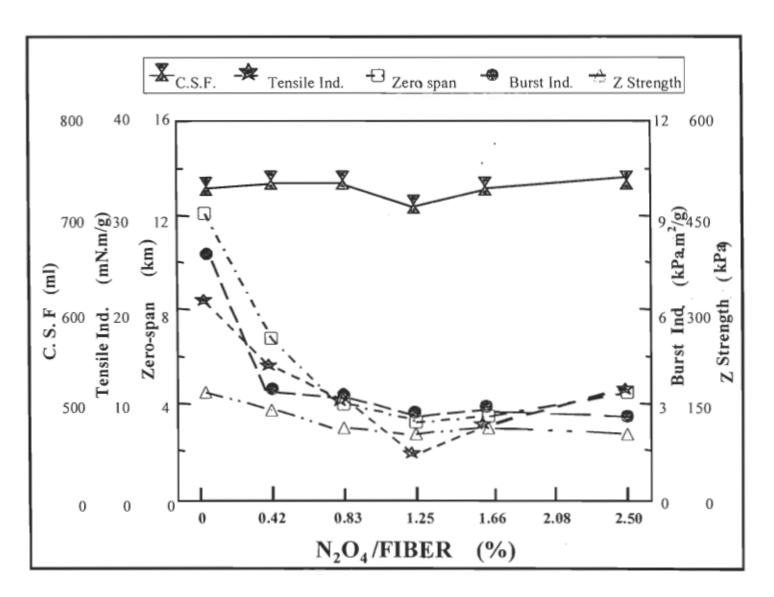
FIGURE 4.83 The variation of CSF, tensile index, zero span, burst index, and z strength of the oxidised softwood bleached kraf fibres as a function of the percentage of N<sub>2</sub>O<sub>4</sub>/fiber.
