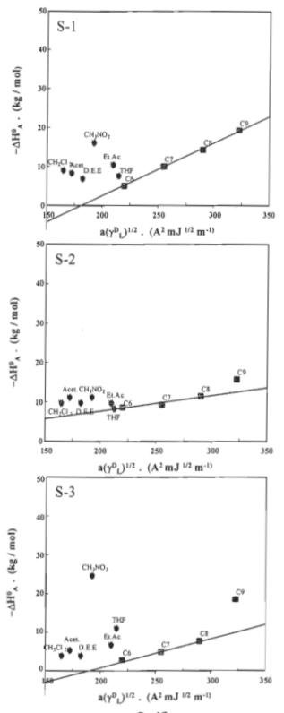
FIGURE A.7 Plot of  $-\Delta H_A$  versus  $a(\gamma^D_L)^{1/2}$  of the alkane and polar probes of the oxidised softwood bleached kraft fibres at N<sub>2</sub>O<sub>4</sub>/fibre of 0.83% (S-1) ,1.25% (S-2) and 1.66% (S-3).
