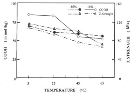
FIGURE 4.6 COOH and z strength as a function of ambient temperature during oxidation by N<sub>2</sub>O<sub>4</sub> at 10% and 35% pulp consistency (2.6 ml/min, 120 min).
