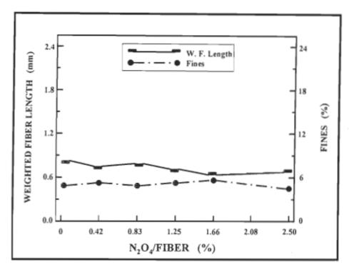
FIGURE 4.82 The variation of the weighted average fibre length and percentage of fines of the oxidised bleached kraft aspen as a function of percentage of N<sub>2</sub>O<sub>4</sub>/fiber.
