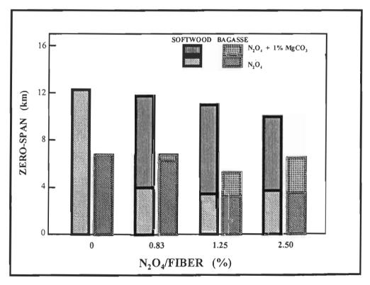
FIGURE 4.94 The effect of the addition 1.0 % MgCO<sub>3</sub> on zero-span during oxidation by N<sub>2</sub>O<sub>4</sub>.
