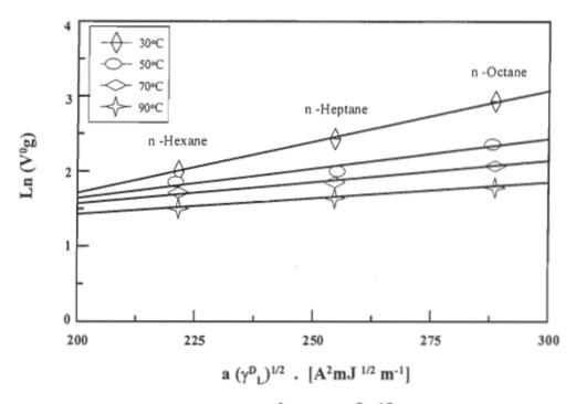
FIGURE 4.48 Linearity between  $\ln{(V^0_g)}$  and  $a(\gamma^D_L)^{1/2}$  for the number of carbons of the alkane probes of the untreated bleached kraft bagasse fibres.
