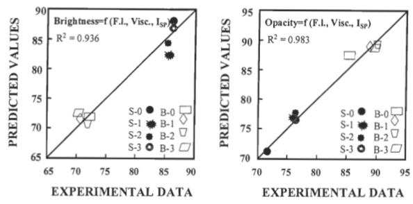
FIGURE 4.107 &4.108 Correlation between the experimental and predicted values of the brightness (Fig. 4.107) and the opacity (Fig.4.108) of softwood and bagasse fibres oxidised by N<sub>2</sub>O<sub>4</sub> in the presence of MgCO<sub>3</sub>.
