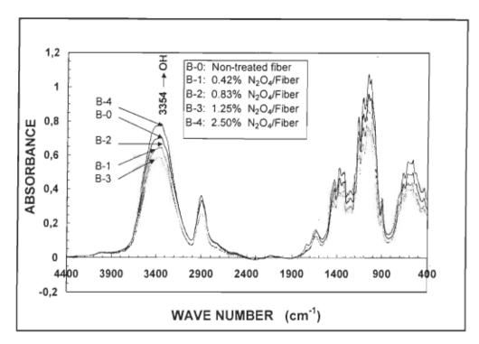
FIGURE 4.26 FTIR absorbance peaks of oxidised bleached kraft bagasse fibres at different oxidation rates of 0, 0.83, 1.25, 1.66 and 2.50 % N<sub>2</sub>O<sub>4</sub> /fibre.
