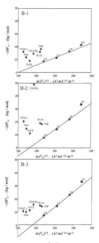
FIGURE A.8 Plot of  $-\Delta H_A$  versus  $a(\gamma^D_L)^{1/2}$  of the alkane and polar probes of the oxidised bagasse bleached kraft fibres at N<sub>2</sub>O<sub>4</sub>/fibre of 0.83% (B-1) ,1.25% (B-2) and 1.66% (B-3).
