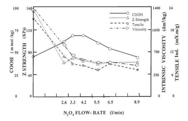
FIGURE 4.1 Fibre characteristics as a function of the gas flow-rate during oxidation by the N<sub>2</sub>O<sub>4</sub> (oxidation time 120 min. temperature 45°C, consistency 10%).
