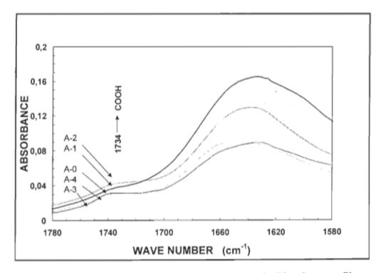
FIGUR 4.29 FTIR absorbance peaks of oxidised bleached kraft aspen fibres at different oxidation rates (0, 0.83, 1.25, 1.66 and 2.50 %N<sub>2</sub>O<sub>4</sub>/fiber (Enlarged for 1580-1780 cm<sup>-1</sup>).
