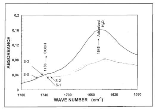
FIGURE 4.31 FTIR absorbance peaks of oxidised blleached kraft softwood fibres at oxidation rates of 0, 0.83, 1.25 and 2.50 %N<sub>2</sub>O<sub>4</sub>/fiber + 1% MgCO<sub>3</sub> (Enlarged for 1580-1780 cm<sup>-1</sup>).
