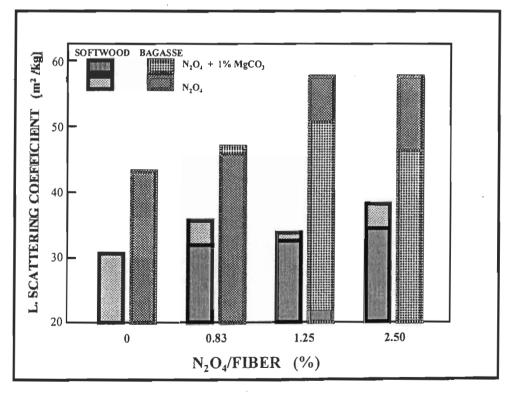
FIGURE 4.98 The effect of the addition 1% MgCO<sub>3</sub> during oxidation by N<sub>2</sub>O<sub>4</sub> on light scattering coefficient.
