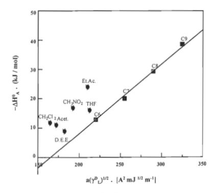
FIGURE 4.63 Plot of  $-\Delta H_A$  versus a  $(\gamma^D_L)^{1/2}$  of the alkane and polar probes of the oxidised bleached kraft aspen fibres at 2.5%  $N_2O_4$ /fibre.
