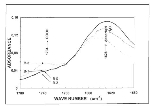
FIGURE 4.33 FTIR absorbance peaks of oxidised bleached kraft bagasse fibres at oxidation rates of 0, 0.83, 1.25 and 2.50 %N<sub>2</sub>O<sub>4</sub>/fibre + 1% MgCO<sub>3</sub> (Enlarged for 1580-1780 cm<sup>-1</sup>).
