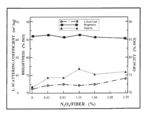
FIGURE 4.86 Brightness, opacity and light scattering coefficient of the oxidised softwood fibres as a function of the percentage of N<sub>2</sub>O<sub>4</sub>/fiber.
