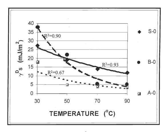
FIGURE A.13 Variations in the value of  $\gamma^D_S$  as a function of the temperature of the IGC column for the untreated softwood (S-0), bagasse (B-0) and aspen (A-0) fibres.
