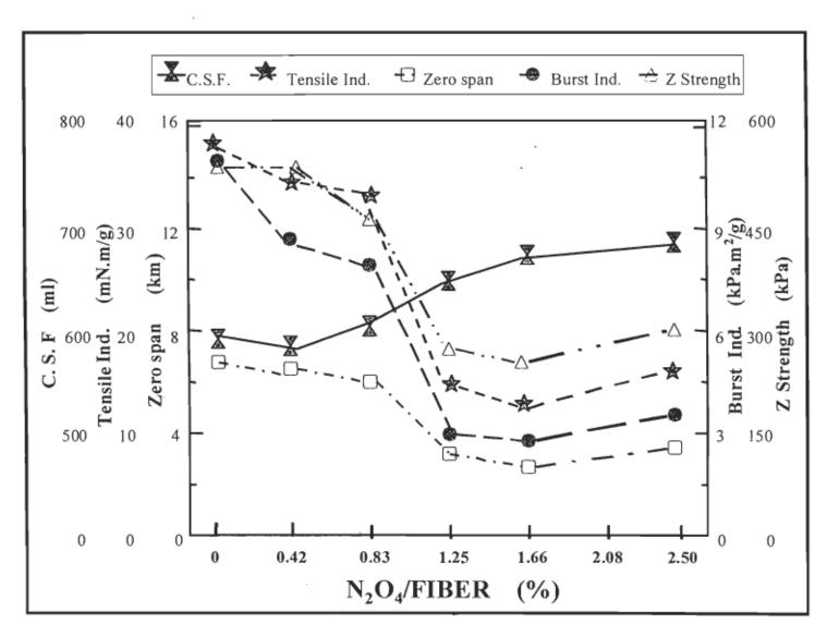
FIGURE 4.84 The variation of CSF, tensile index, zero span, burst index, and z strength of the oxidised bagasse bleached kraft fibres as a function of the percentage of N<sub>2</sub>O<sub>4</sub>/fiber.
