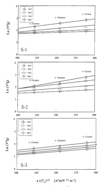
FIGURE A.1 Linearity between  $\ln(V^0_g)$  and  $a(\gamma)^{1/2}$  for the number of carbon of the alkane probes of the oxidised softwood bleached kraft fibres with  $N_2O_4$  /fibre of 0.8% (S-1), 1.25% (S-2) and 1.66% (S-3).
