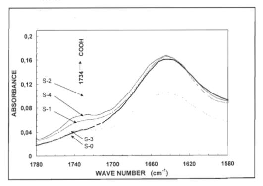
FIGURE 4.25 FTIR absorbance peaks of oxidised bleached kraft softwood fibres at different oxidation rates of 0, 0.83, 1.25, 1.66 and 2.50 % N<sub>2</sub>O<sub>4</sub> /fibre (Enlarged for 1580-1780 cm<sup>-1</sup>).
