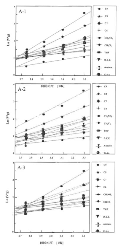
FIGURE A.6 Linearity of  $ln(V^0{}_g)$  versus the inverse increase in the temperature of the alkane probes of the oxidised aspen fibres with  $N_2O_4$  /fibre of 0.83% (A-1), 1.25% (A-2) and 1.66% (A-3).
