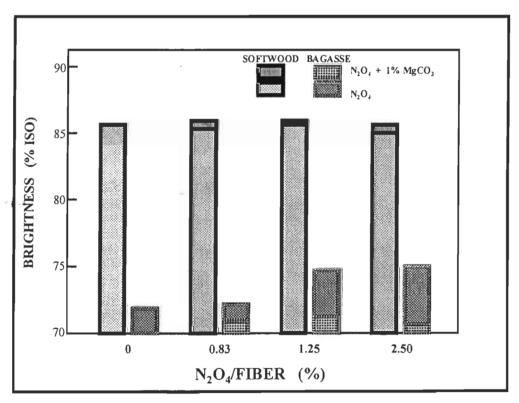
FIGURE 4.96 The effect of the addition 1.0 % MgCO<sub>3</sub> during oxidation by N<sub>2</sub>O on brightness.
