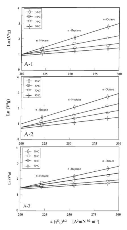
FIGURE A.3 Linearity between  $ln(V_g^0)$  and  $a(\gamma)^{1/2}$  for the number of carbon of the alkane probes of the oxidised aspen bleached kraft fibres with  $N_2O_4$ /fibre of 0.83% (A-1), 1.25% (A-2) and 1.66% (A-3).
