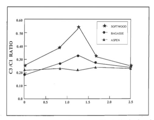
FIGURE 4.38 The effect of N<sub>2</sub>O<sub>4</sub> oxidation of bleached kraft softwood, bagasse and aspen fibres on C3/C1 ratio.
