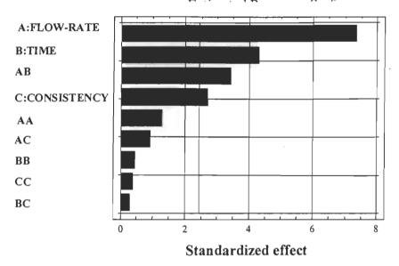
FIGURE 4.13 The standardised Pareto chart of viscosity for the oxidation factors.
