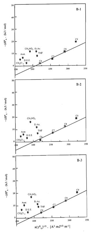
FIGURE 4.74 Plot of  $-\Delta H_A$  versus  $a(\gamma^D_L)^{1/2}$  for the bagasse bleached kraft fibres oxidised with 0.83%, 1.25% and 2.5 %  $N_2O_4$  (B-1, B-2 and B-3) plus 1% MgCO<sub>3</sub>.
