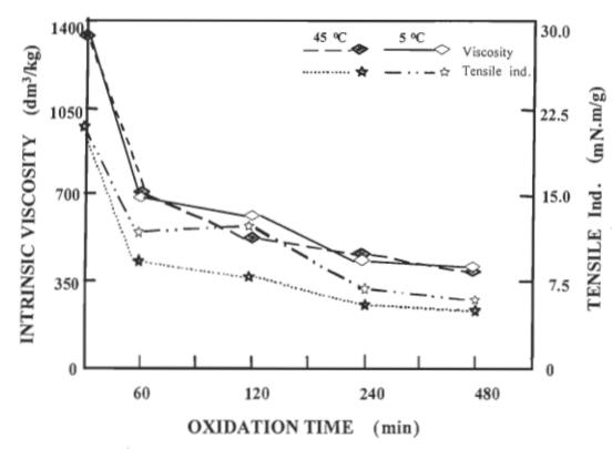
FIGURE 4.2 Intrinsic viscosity and tensile index as a function of the time of oxidation by N<sub>2</sub>O<sub>4</sub> at 5°C and 45 °C (10% pulp consistency).
