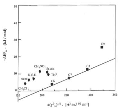
FIGURE 4.59 Plot of  $-\Delta H_A$  versus a  $(\gamma^D_L)^{1/2}$  of the alkane and polar probes of the oxidised bleached kraft softwood fibres at 2.5%  $N_2O_4$ /fibre.
