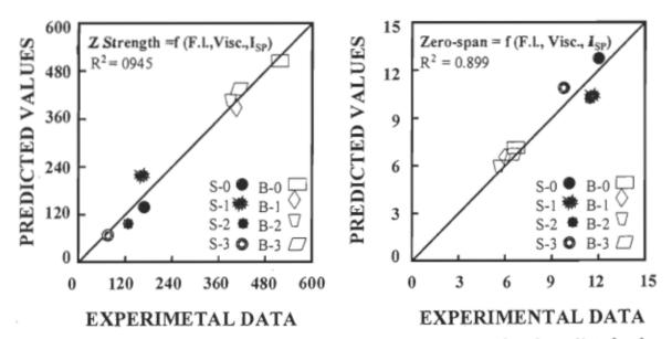
FIGURE 4.105 & 4.106 Correlation between the experimental and predicted values of the z strength (Fig. 4.105) and the zero span (Fig. 4.106) of softwood and bagasse fibres. These were oxidised by N<sub>2</sub>O<sub>4</sub> in presence of MgCO<sub>3</sub>.
