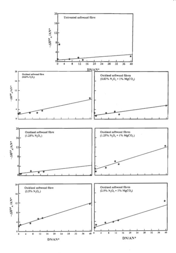
FIGURE 4.75 Plot of ΔH<sup>SP</sup><sub>A</sub>/AN\* versus DN/AN\* for untreated and oxidised softwood fibres without MgCO<sub>3</sub> (left side) and in presence of MgCO<sub>3</sub> (right side).
