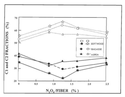
FIGURE 4.37 The effect of N<sub>2</sub>O<sub>4</sub> oxidation of bleached kraft softwood, bagasse and aspen fibres on C1 and C2 fractions.
