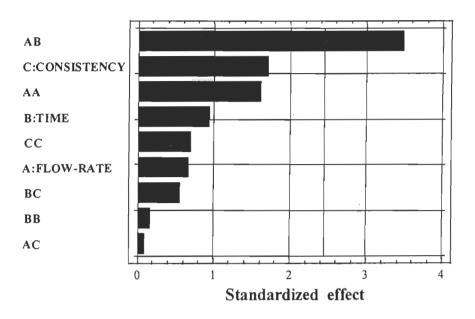
FIGURE 4.11 Standardised Pareto chart of carboxyl content for the oxidation factors.
