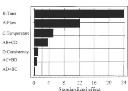
FIGURE 4.8 Standardised Pareto chart for the viscosiy of oxidised fibres of bleached kraft softwood.
