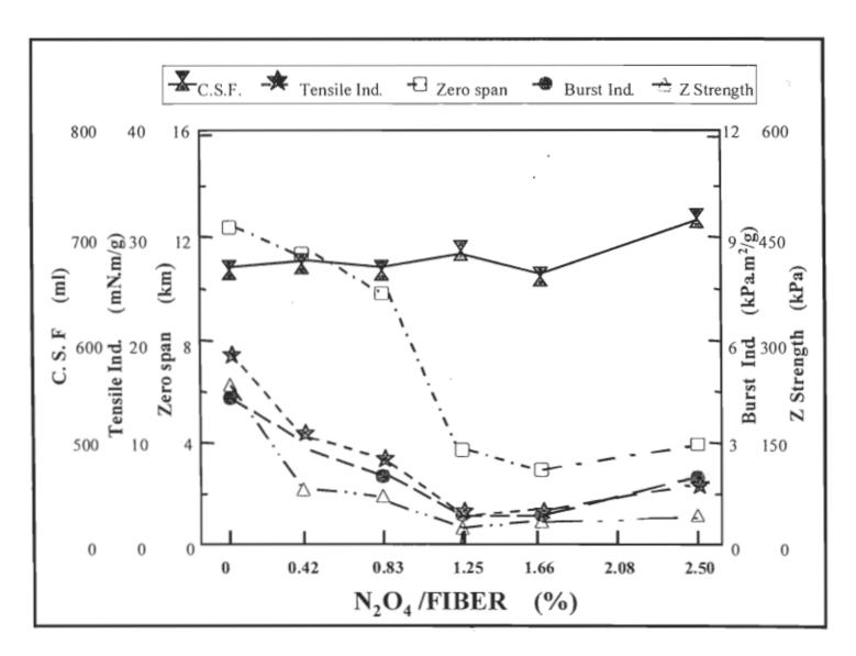
FIGURE 4.85 The variation of CSF, tensile index, zero span, burst index, and z strength of the oxidised aspen bleached kraft fibres as a function of the percentage of N<sub>2</sub>O<sub>4</sub>/fiber.
