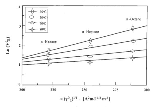
FIGURE 4.50 Linearity between  $\ln{(V^0_g)}$  and  $a(\gamma^D_L)^{1/2}$  for the number of carbons of the alkane probes of the untreated bleached kraft aspen fibres.
