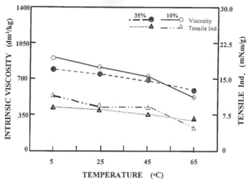
FIGURE 4.5 Intrinsic viscosity and tensile index as a function of ambient temperature during oxidation by N<sub>2</sub>O<sub>4</sub> at 10% and 35 % pulp consistency (2.6 ml/min, 120 min).
