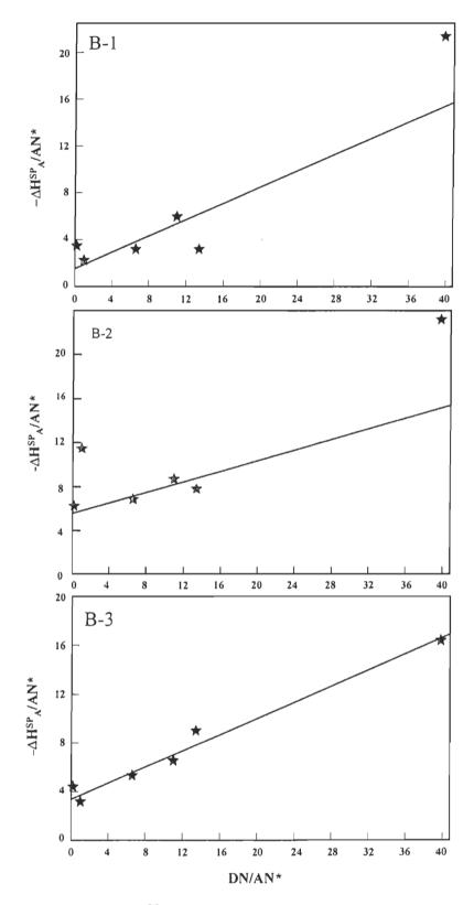
FIGURE A.11 Plot of  $-\Delta H^{SP}_A/AN^*$  versus DN/AN\* for the oxidised bagasse bleached kraft fibres at N<sub>2</sub>O<sub>4</sub>/fibre of 0.83% (B-1), 1.25% (B-2) 1.66% (B-3), allowing the determination of  $K_A$  and  $K_B$ .
