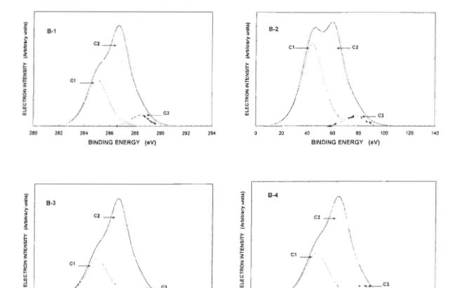
FIGURE 4.35 C (1s) peaks obtained from ESCA spectra for bagasse oxidized by  $N_2O_4$  at oxidation rates of 0.0% (B-0), 0.83% (B-1), 1.25% (B-2), 1.66% (B-3) and 2.50% (B-4).
