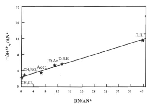
FIGURE 4.65 Plot of  $-\Delta H^{SP}_A/AN^*$  versus DN/AN\* for the oxidised bleached kraft softwood fibres with 2.5 % N<sub>2</sub>O<sub>4</sub> allowing the determination of the acceptor constant,  $K_A$  and donor constant,  $K_B$ .
