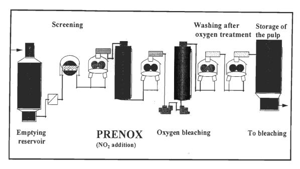
FIGURE 2.9 Installation diagram of Prenox (17).
