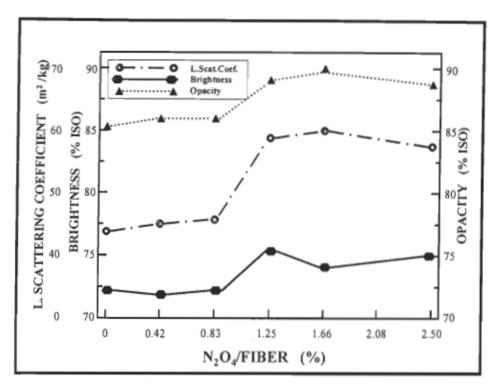
FIGURE 4.87 Brightness, opacity and light scattering coefficient of the oxidised bagasse fibres as a function of the percentage of N<sub>2</sub>O<sub>4</sub>/fiber.
