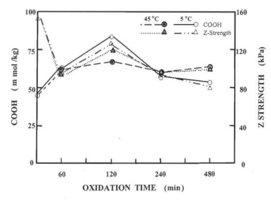
FIGURE 4.3 COOH and z strength as a function of the time of oxidation by N<sub>2</sub>O<sub>4</sub> at 5 °C and 45°C (10% pulp consistency)..
