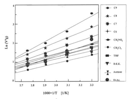
FIGURE 4.56 Linearity of  $\ln{(V^0}_g)$  versus the inverse temperature of injection of the alkane and polar probes of the untreated aspen fibres.
