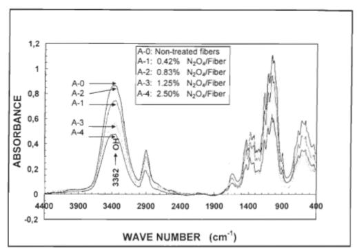
FIGUR 4.28 FTIR absorbance peaks of oxidised bleached kraft aspen fibres at different oxidation rates (0, 0.83, 1.25, 1.66 and 2.50 %N<sub>2</sub>O<sub>4</sub> /fiber).
