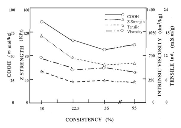
FIGURE 4.4 Fibre characteristics as a function of the pulp consistency during oxidation by N<sub>2</sub>O<sub>4</sub> (2.6 ml/min, 120 min, 5°C).
