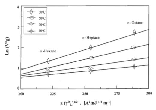
FIGURE 4.49 Linearity between  $\ln (V_g^0)$  and  $a(\gamma_L^0)^{1/2}$  for the number of carbons of the alkane probes of the bleached kraft bagasse fibres with 2.5%N<sub>2</sub>O<sub>4</sub>.
