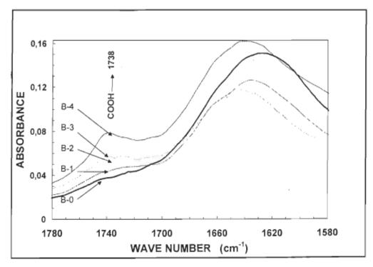
FIGURE 4.27 FTIR absorbance peaks of oxidised bleached kraft bagasse fibres at different oxidation rates of 0, 0.83, 1.25, 1.66 and 2.50% N<sub>2</sub>O<sub>4</sub> /fibre (Enlarged for 1580-1780-cm<sup>-1</sup>).
