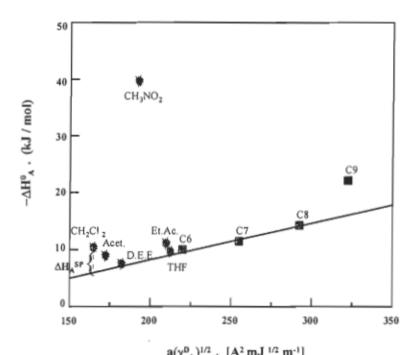
$a(\gamma^D_{\ 1})^{1/2}$ . [A<sup>2</sup> mJ  $^{1/2}$  m·1] FIGURE 4.58 Plot of  $-\Delta H_A$  versus a  $(\gamma^D_{\ L})^{1/2}$  of the alkane and polar probes of the untreated bleached kraft softwood fibres.
