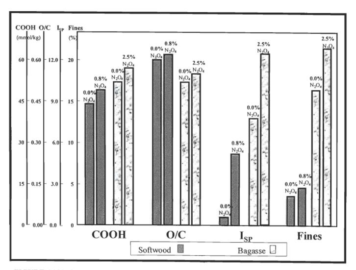
FIGURE 4.101 Factors affecting bonding strength of softwood and bagasse fibres oxidised by  $N_2O_4$  in presence of 1% MgCO<sub>3</sub>.
