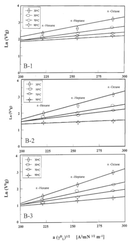
FIGURE A.2 Linearity between  $\ln(V_g^0)$  and  $a(\gamma)^{1/2}$  for the number of carbon of the alkane probes of the oxidised bagasse bleached kraft fibres with  $N_2O_4$ /fibre of 0.83% (B-1), 1.25% (B-2) and 1.66% (B-3).
