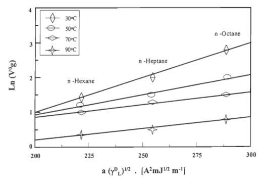
FIGURE 4.51 Linearity between ln  $(V_g^0)$  and  $a(\gamma_L^0)^{1/2}$  for the number of carbons of the alkane probes of the bleached kraft aspen fibres with 2.5%  $N_2O_4$ .
