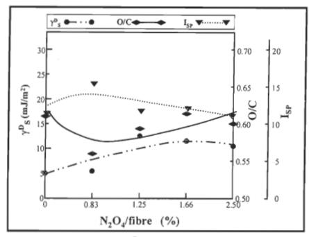
FIGURE 4.72 The relation between γ<sup>D</sup><sub>S</sub> with the O/C ratio and the I<sub>SP</sub> as the function of the percentage of N<sub>2</sub>O<sub>4</sub>/fibre for the aspen oxidised fibres.
