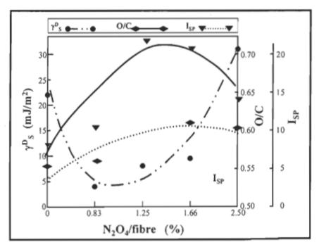
FIGURE 4.71 The relation between  $\gamma^D_S$  with the O/C ratio and the  $I_{SP}$  as the function of the percentage of  $N_2O_4$ /fibre for the bagasse oxidised fibres.
