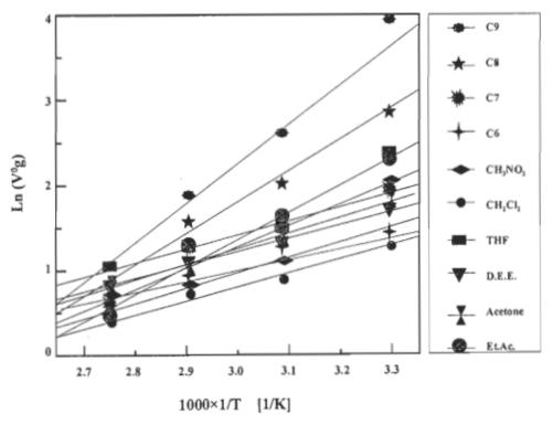
FIGURE 4.57 Linearity of  $\ln{(V^0}_g)$  versus the inverse temperature of injection of the alkane and polar probes of the oxidised aspen fibres with 2.5%  $N_2O_4$ .
