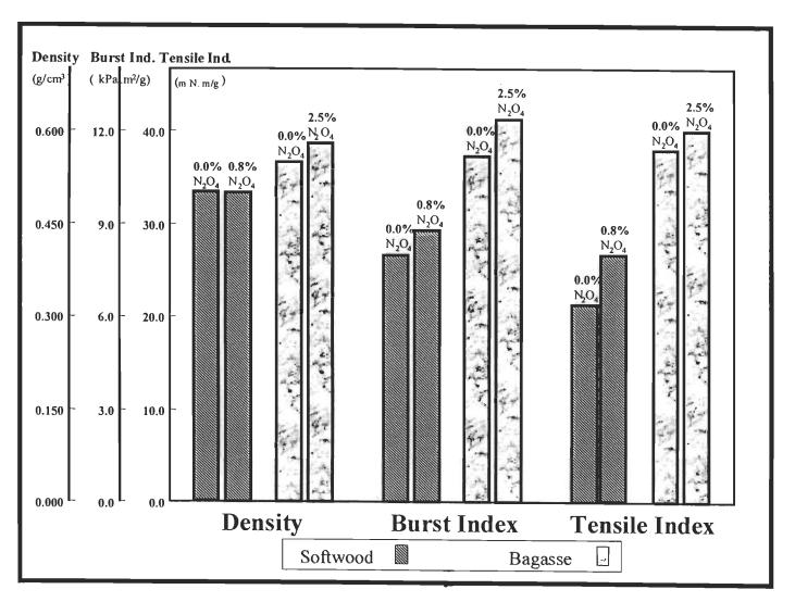
FIGURE 4.102 Strength properties improvement of the sheets made by the softwood and bagasse fibres oxidised by N<sub>2</sub>O<sub>4</sub> in presence of 1% MgCO<sub>3</sub>.
