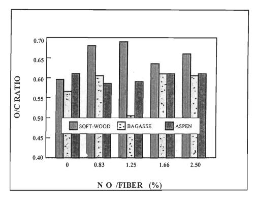
FIGURE 4.39 The effect of N<sub>2</sub>O<sub>4</sub> oxidation of the bleached kraft fibres of softwood, bagasse and aspen on the O/C ratio.
