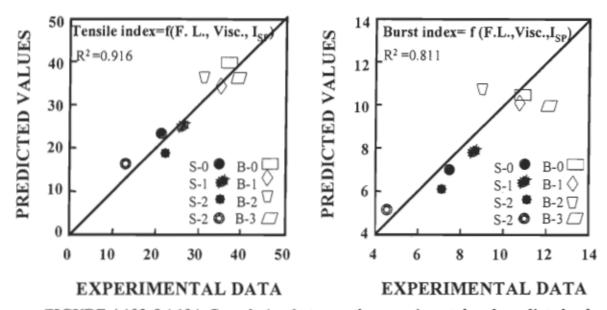
FIGURE 4.103 &4.104 Correlation between the experimental and predicted values of the tensile index (Fig. 4.103) and the burst index (Fig. 4.104) of softwood and bagasse fibres oxidised by N<sub>2</sub>O<sub>4</sub> in the presence of MgCO<sub>3</sub>
