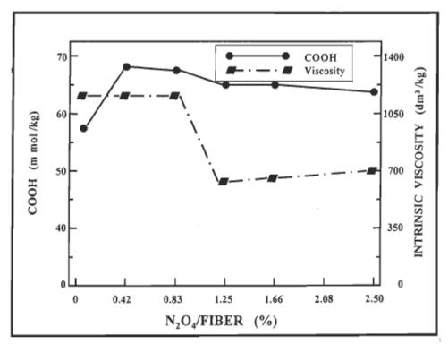
FIGURE 4.79 The variations of intrinsic viscosity and COOH of the oxidised bleached kraft aspen fibres as a function of the percentage of N<sub>2</sub>O<sub>4</sub>/fiber.
