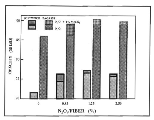
FIGURE 4.97 The effect of the addition 1% MgCO<sub>3</sub> during oxidation by N<sub>2</sub>O<sub>4</sub> on opacity.
