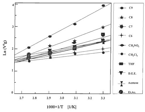
FIGURE 4.54 Linearity of  $\ln{(V^0_g)}$  versus the inverse temperature of injection of the alkane and polar probes of the untreated bagasse fibres.
