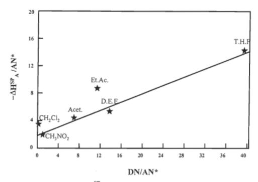
FIGURE 4.68 Plot of  $-\Delta H^{SP}_A/AN^*$  versus DN/AN\* for the untreated bleached kraft aspen fibres allowing the determination of the acceptor constant,  $K_A$  and donor constant,  $K_B$ .
