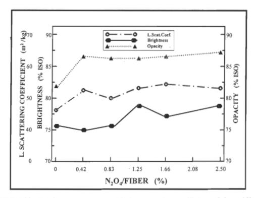
FIGURE 4.88 Brightness, opacity and light scattering coefficient of the oxidised aspen fibres as a function of the percentage of N<sub>2</sub>O<sub>4</sub>/fiber.
