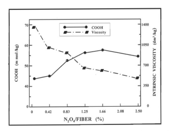
FIGURE 4.77 The variations of intrinsic viscosity and COOH of the oxidised bleached kraft softwood fibres as a function of the percentage of N<sub>2</sub>O<sub>4</sub>/fiber.
