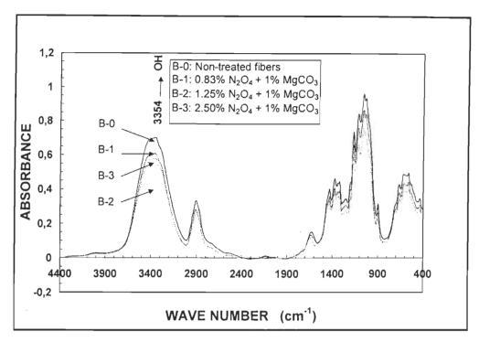
FIGURE 4.32 FTIR absorbance peaks of oxidised fibers of bleached kraft bagasse with oxidation rates of 0, 0.83, 1.25 and 2.50  $\%N_2O_4$ /fiber + 1% MgCO<sub>3</sub>.
