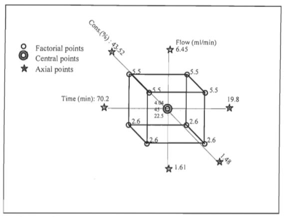
FIGURE. 3.6 A CCD model for the three-variable parameters of the N<sub>2</sub>O<sub>4</sub> oxidation. These are gas flow-rate, oxidation time and pulp consistency, each one at five levels, 3 <sup>4-1</sup>.
