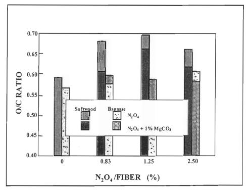
FIGURE 4.45 Plot of O/C ratio of beached kraft fibres of softwood and bagasse versus the  $N_2O_4$  oxidation rate, in presence of 1% MgCO<sub>3</sub>.
