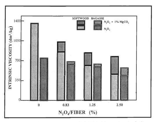
FIGURE 4.89 The effect of the addition of 1.0 % MgCO<sub>3</sub> on viscosity during oxidation by N<sub>2</sub>O<sub>4</sub>.
