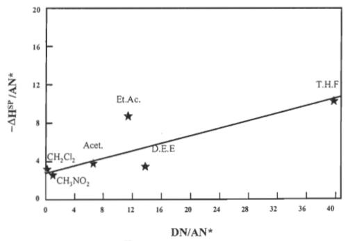
FIGURE 4.69 Plot of  $-\Delta H^{SP}_A/AN^*$  versus DN/AN\* for the oxidised bleached kraft aspen fibres with 2.5 % N<sub>2</sub>O<sub>4</sub> allowing the determination of the acceptor constant,  $K_A$  and donor constant,  $K_B$ .
