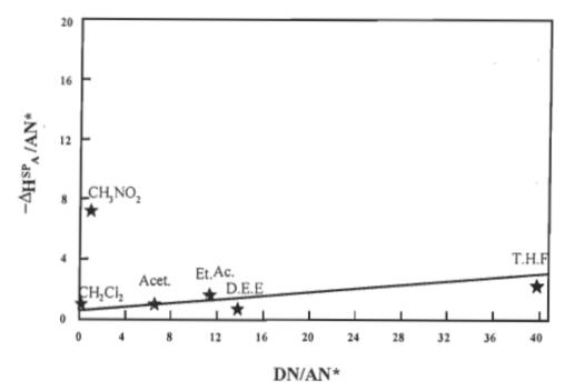
FIGURE 4.64 Plot of  $-\Delta H^{SP}_A/AN^*$  versus DN/AN\* for the untreated bleached kraft softwood fibres allowing the determination of the acceptor constant,  $K_A$  and donor constant,  $K_B$ .
