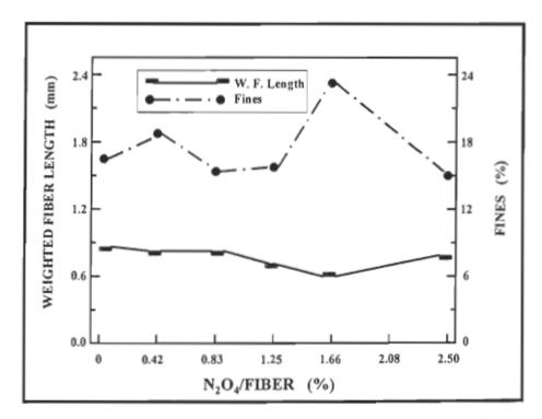
FIGURE 4.81 The variation of the weighted average fibre length and percentage of fines of the oxidised bleached kraft bagasse as a function of percentage of N<sub>2</sub>O<sub>4</sub>/fiber.
