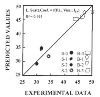
FIGURE 4.109 Correlation between the experimental and predicted values of the light scattering coefficient of softwood and bagasse fibres oxidised by N<sub>2</sub>O<sub>4</sub> in the presence of MgCO<sub>3</sub>.
