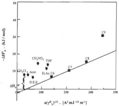
FIGURE 4.60 Plot of  $-\Delta H_A$  versus a  $(\gamma^D_L)^{1/2}$  of the alkane and polar probes of the untreated bleached kraft bagasse fibres.
