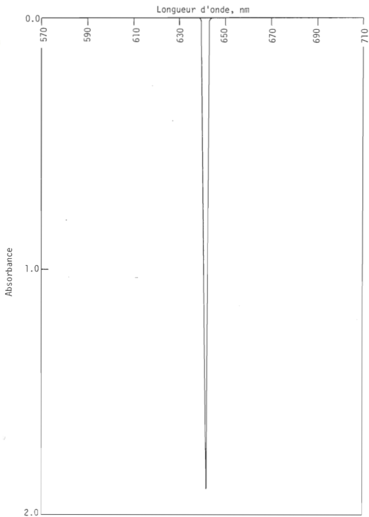
FIGURE 2.1.5: Spectre de transmission du filtre Oriel RG 632.8
