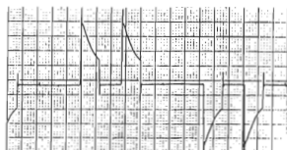
ac line current; 0.5 A/div, 1 ms/div
