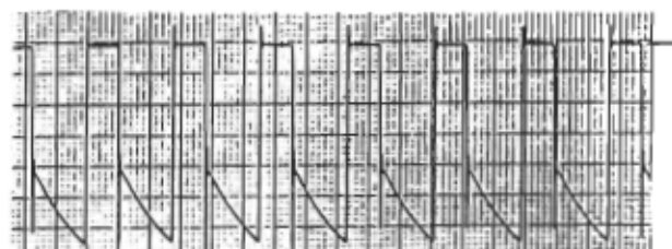
dc-terminal voltage; 25 V/div, 1 ms/div.
