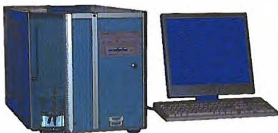
Figure 2: Morpho Wall Thickness measurement device (CTP/TechPap)
