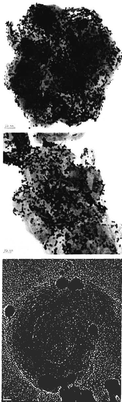
Fig. 3. HRTEM images of Pt nanoparticles supported in functionalized CNS sample F.
