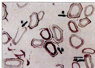
Fig. 4: Cross-section view of TMP fibers
