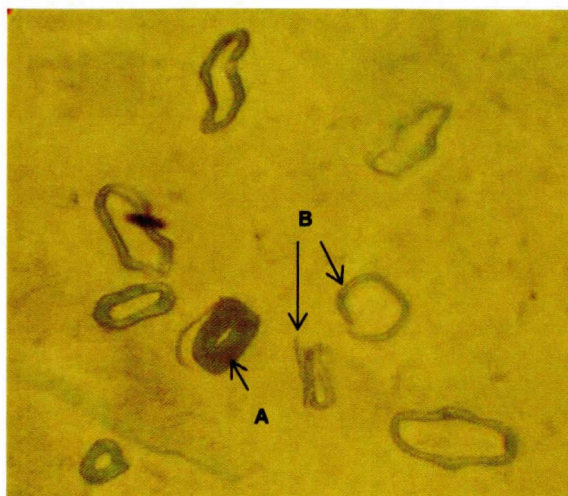
Figure 8.44 Cell wall failure of EW and LW fibres in refining
