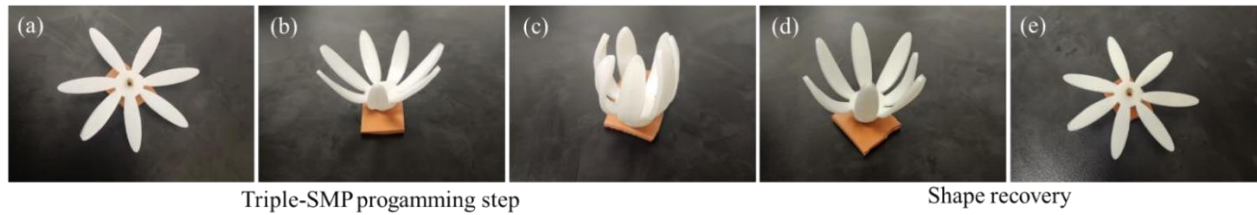
Figure 4.10: 7 petals flower configuration of triple-shape memory based on 4D printing of PLA-75/PETG-25 polymer blend: (a) original shape 1; (b) shape 2, blended at 90 °C and cooled to 50 °C; (c) shape 3, blended at 50 °C and cooled to 25 °C; (d) recovered shape 2 after heating at 60 °C; (e) recovered shape 1 after heating to 90 °C.
