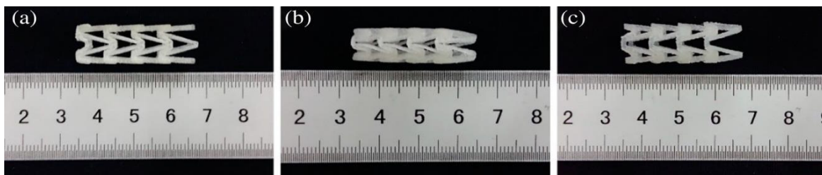
Figure 2.11: Transformation of a 3D-printed stent featuring an arrowhead structure: (a) post-printing, (b) following crimping; (c) after recovery [46, 131].
