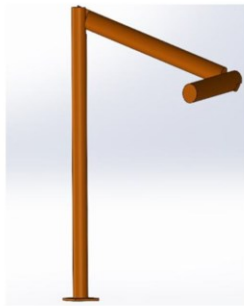
Fig. 7. Simplified SolidWorks model of the ABB IRB 140 robotic arm
