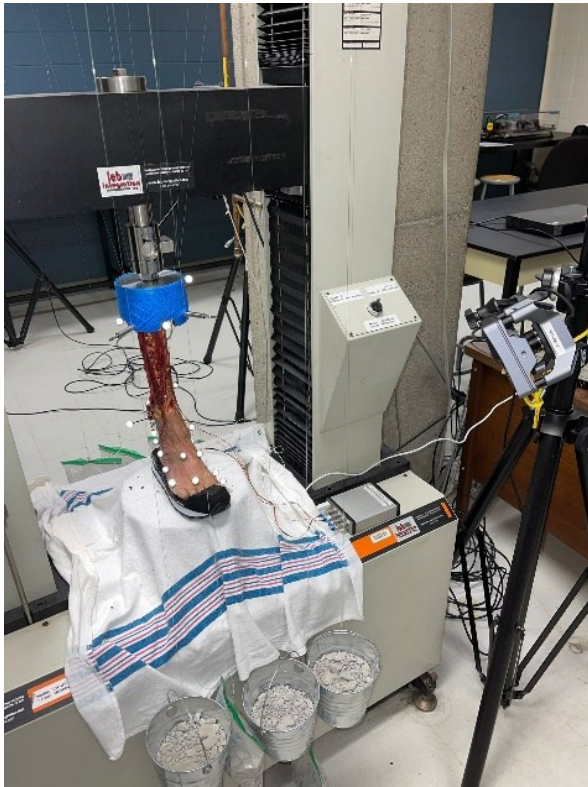
Figure 18 Experimental setup on the mechanical press
