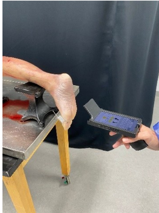
Figure 16 Foot scanning for the design of foot orthoses
