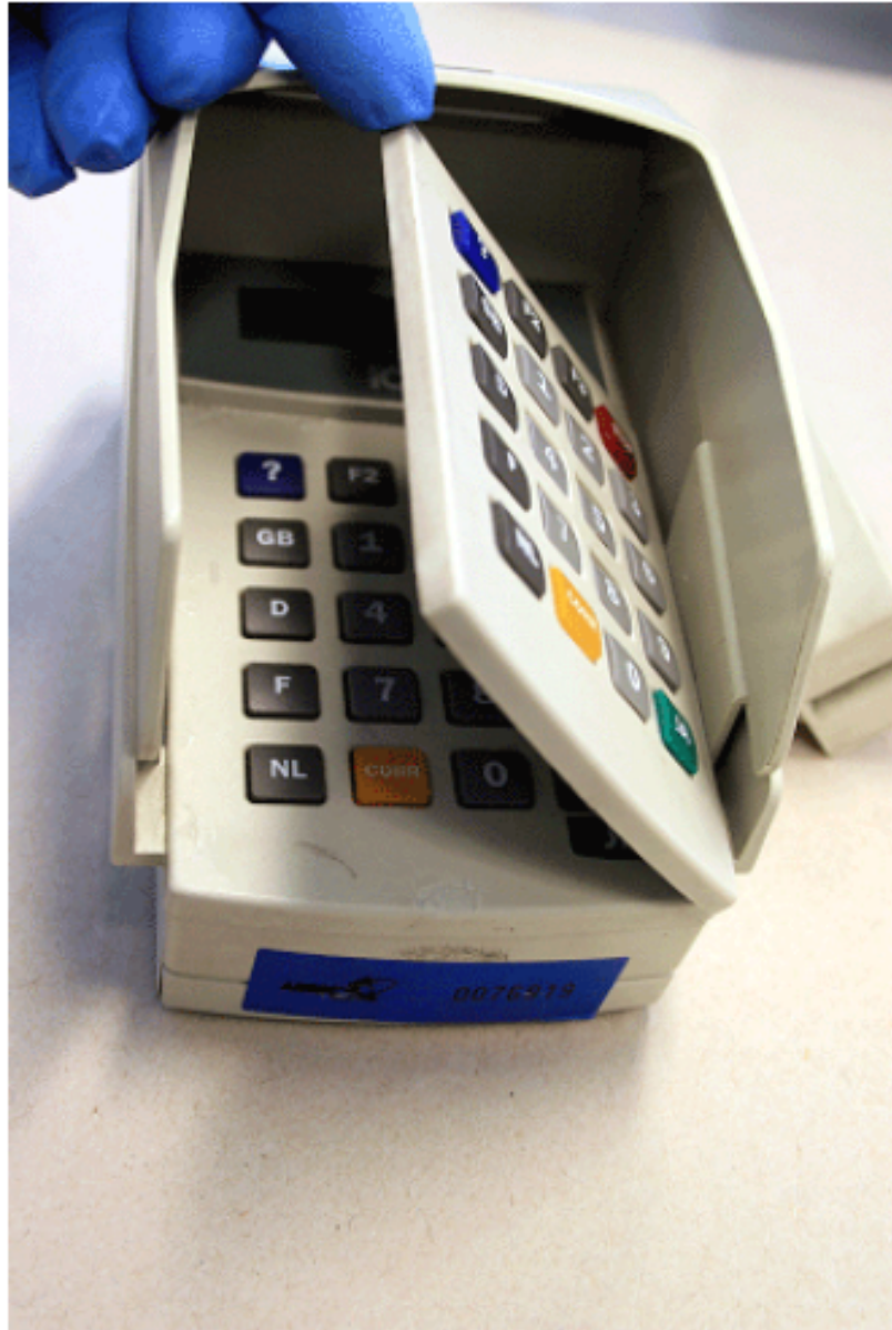
FIGURE 2.1 – Cardblocker PIN reader terminal topper[2]
