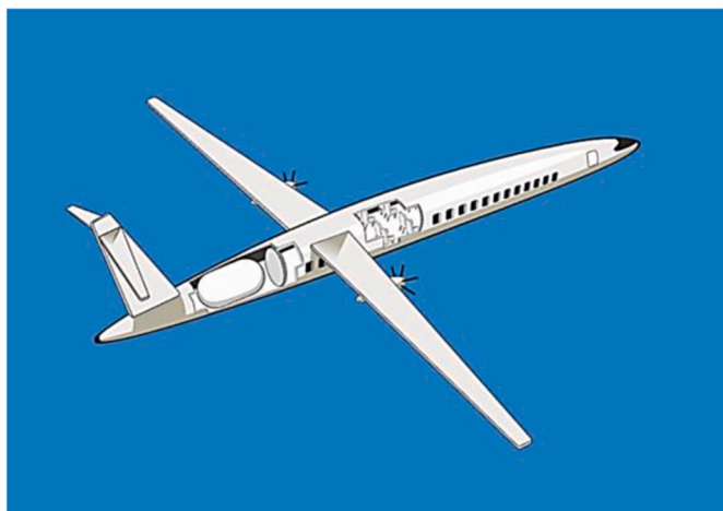
Fig. 35. Schematic diagram for the fuel tank location in a narrow-body LH 2 -powered aircraft [10].
