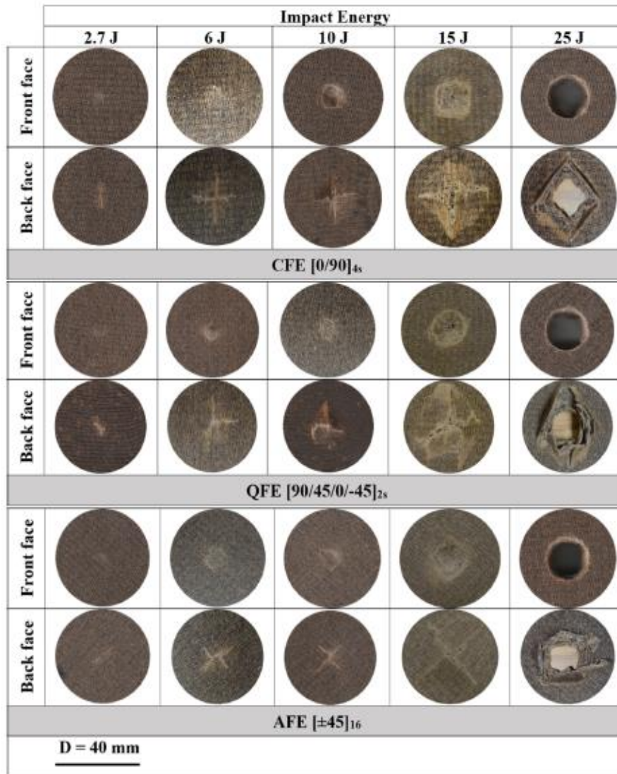
Fig. 8. Visual damage on the front and back faces of impacted specimens at various energy levels.
