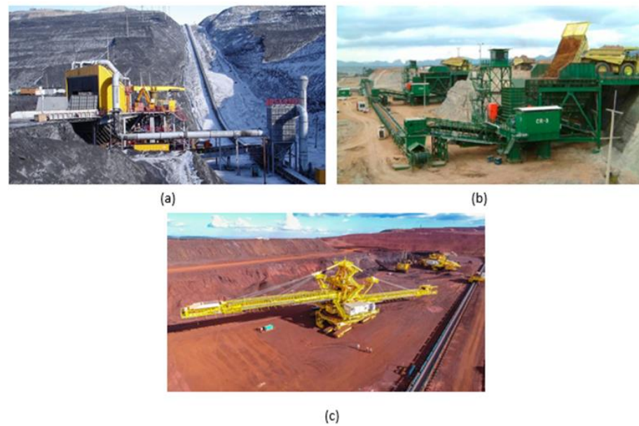
Figure 6. (a) Fixed PCC system, (b) semi-mobile PCC system, and (c) fully mobile PCC system [48].
