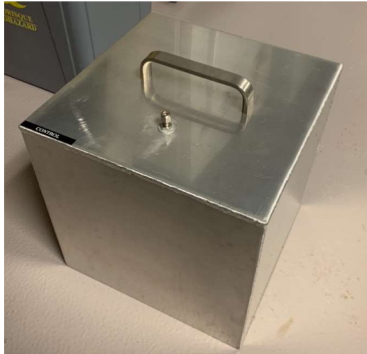
Figure 2.1 Stainless steel hood used to create headspace above samples
