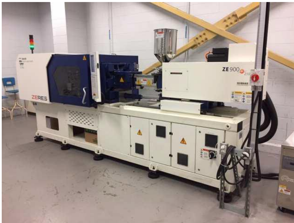
Figure 3.2 Machine de 100 tonnes de, ZE 900 de ZHAFIR Plastics Machinery [14]
