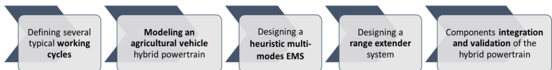
Figure 3-1. General overview of the proposed design process for the off-road agricultural hybrid electric vehicles powertrain.
