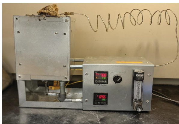
Figure 17 Four à calcination (configuration verticale)
