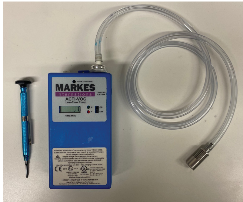
Figure 2.3: ACTI-VOC pump with flat bladed screwdriver used to operate the pump.
