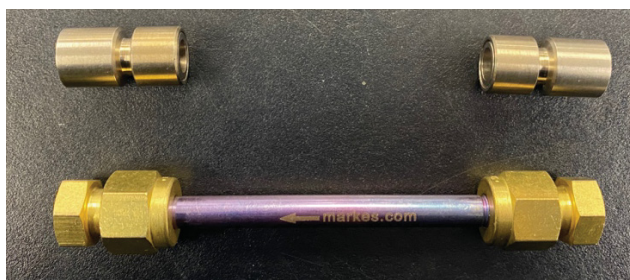
Figure 2.1: Stainless steel sorbent tubes sealed with brass caps (bottom) and diffLock caps (top).
