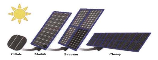
Figure 1.3. Configuration des cellules photovoltaïques [38]
