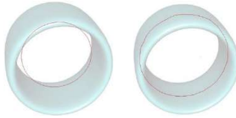
Figure 1.2- The centeredness of the skeleton [2]. Left) the red skeleton out of the object. Right) visually centered skeleton.
