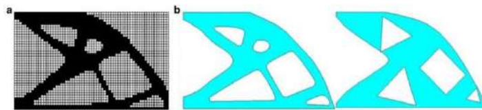
Figure 2.23- a) TO result, b) configuration after image interpretation (middle: IASOS, right: ASOS) [64]
