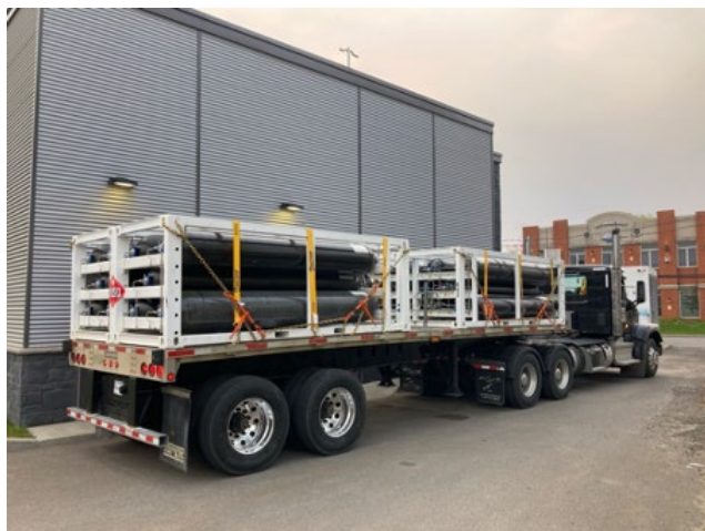
Figure 27 : High-pressure tanks installed on a trailer. Hydrogen capacity of 180 kg at 450 bar. Credit: Harnois Énergies.
