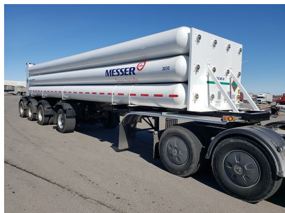
Figure 24 : Low-pressure tube trailer (386 kg of hydrogen at 180 bar) [170].
