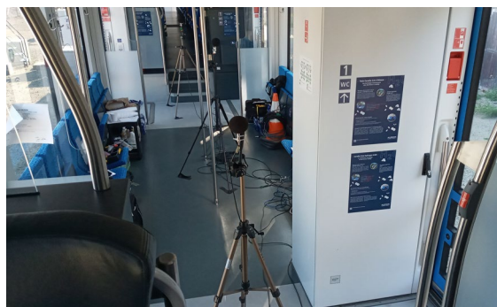
Figure 38 : Photograph of microphones 2, 3, and 4 in the train.
