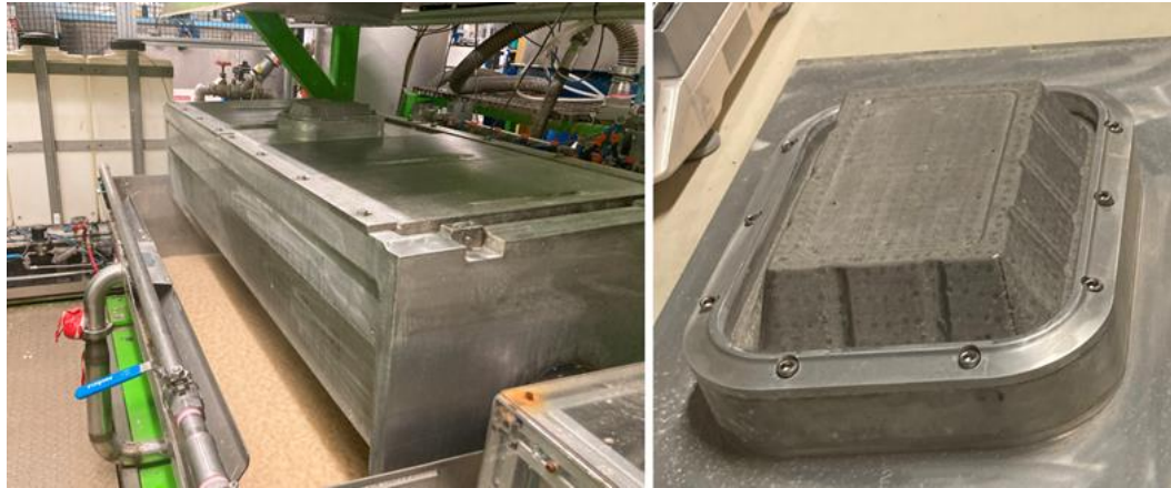
Figure 4-2 : Formation section of the Innofibre's MSIPME – TF-45 industrial machine.
