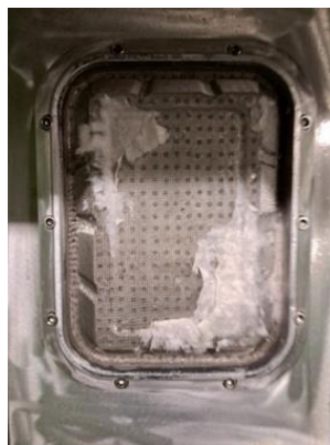
Figure 4-8 : Tray that sticks to the mold during transfer when the drainage time is too high.
