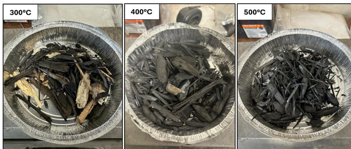
Supplementary figure 11: Extent of carbonization with increase in pyrolysis temperature from 300-500 °C
