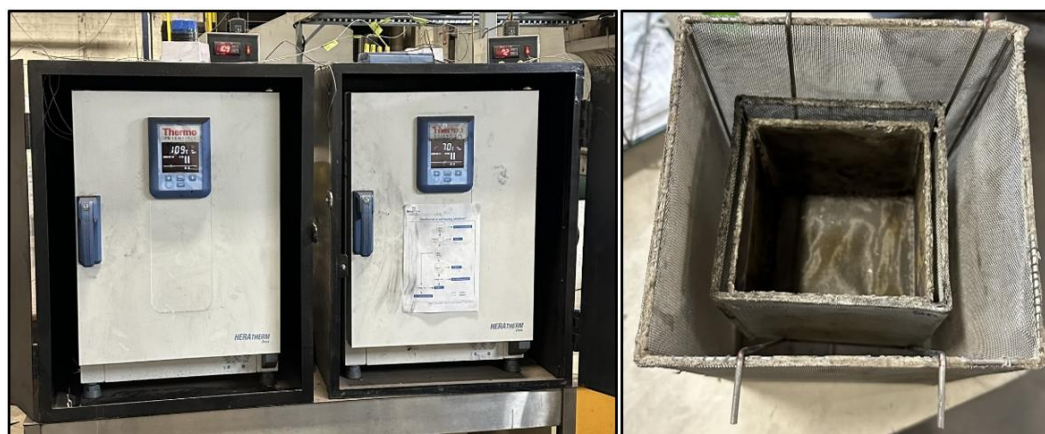
Supplementary figure 19: Biochar basket self-heating set-up with adiabatic ovens
