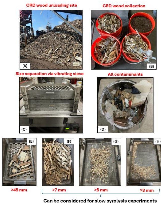
Figure 3: CRD wood sorting, size-separation, and contaminant removal
