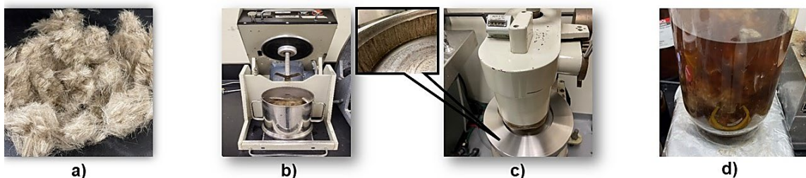
Figure 1. Steps in the mechanical and alkaline pretreatment process of the short flax fibres. a) Short flax fibres, b) Standard disperser, c) PFI refining mill and d) Alkaline treatment of fibrillated fibres.
