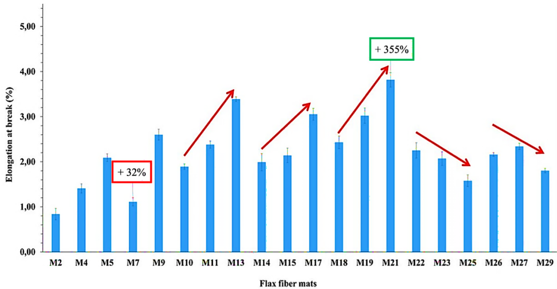
Figure 5.9 Elongation at break (%) of flax mat made from different fiber types.
