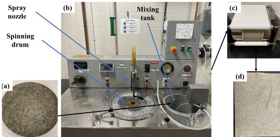
Figure 3. Overview of the flax fiber mat preparation process. (a) A sample of the initial fiber-water slurry used for mat formation. (b) The dynamic forming machine. (c) The E-100 drum dryer employed for drying the formed mats. (d) An example of the finished flax fiber mat.
