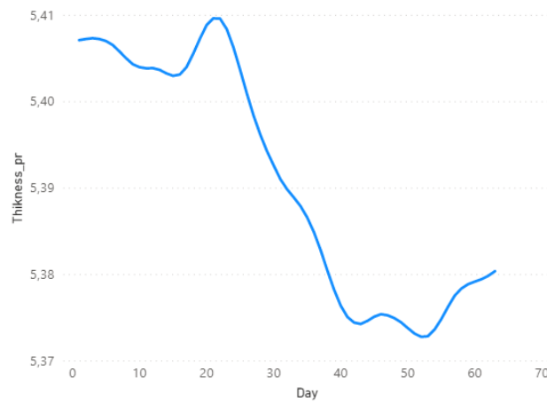
Fig. 3 Measurement of the average thickness predicted by the LSTM model
