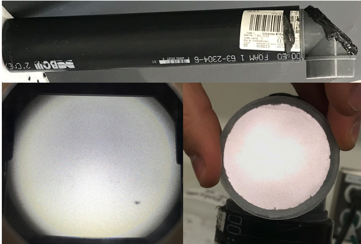
Figure 55: Lighting apparatus made from an ABS 1.5 inch plumbing tube (top). Illumination comparison between a ZEISS Stemi 305 compact stereo microscope backlight (left) and custom made CeSAR's ABS tube (right).
