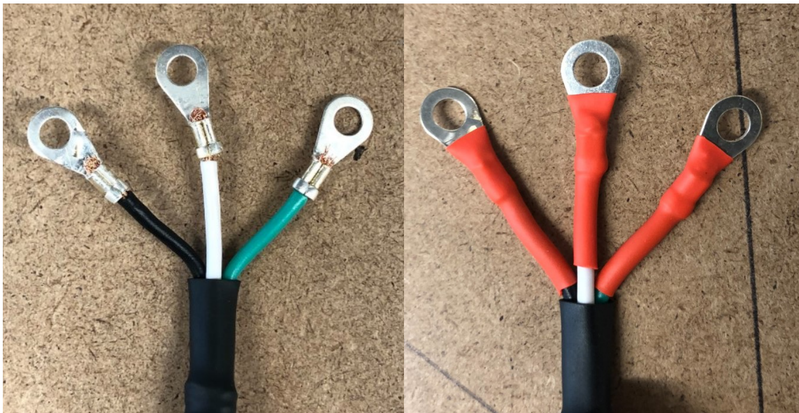
Figure 50: End wires ring terminal connectors used to power the motors and fan's power supply.
