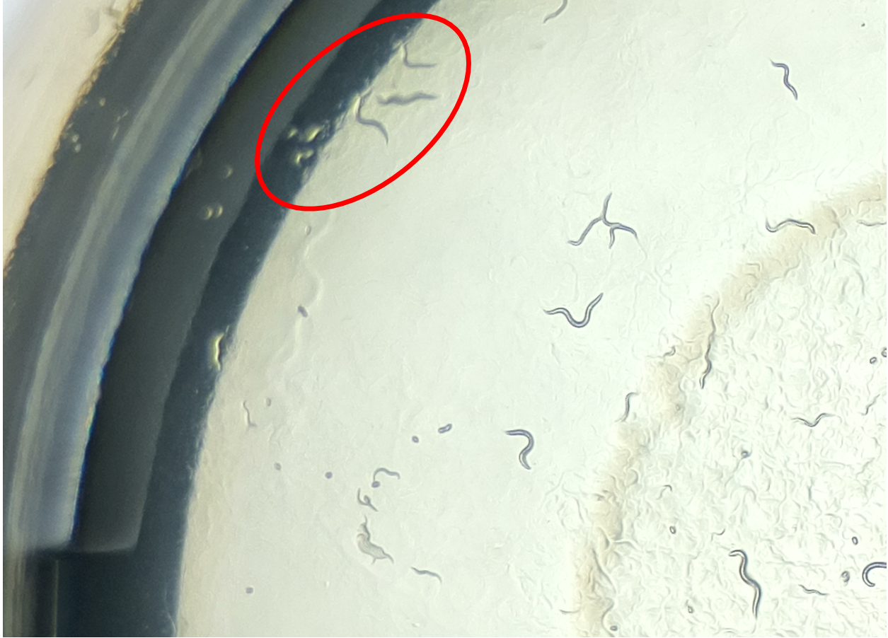
Figure 41: Meniscus formation in untreated well, causing out-of-focus edge and optical blur. The worms and eggs near the center of the well (i.e. on the bacterial lawn) are much more in focus than those closer to the edge, circled in red.
