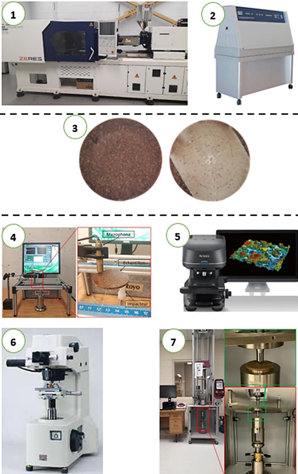
Figure 7. 2. The equipment and samples used: 1- injection moulding machine; 2- accelerated weathering machine; 3- an unaged and aged PP30-F samples example; 4- impulse excitation technic device; 5- 3d confocal microscopy device; 6- Hardness machine; 7- Drop weight impact machine
