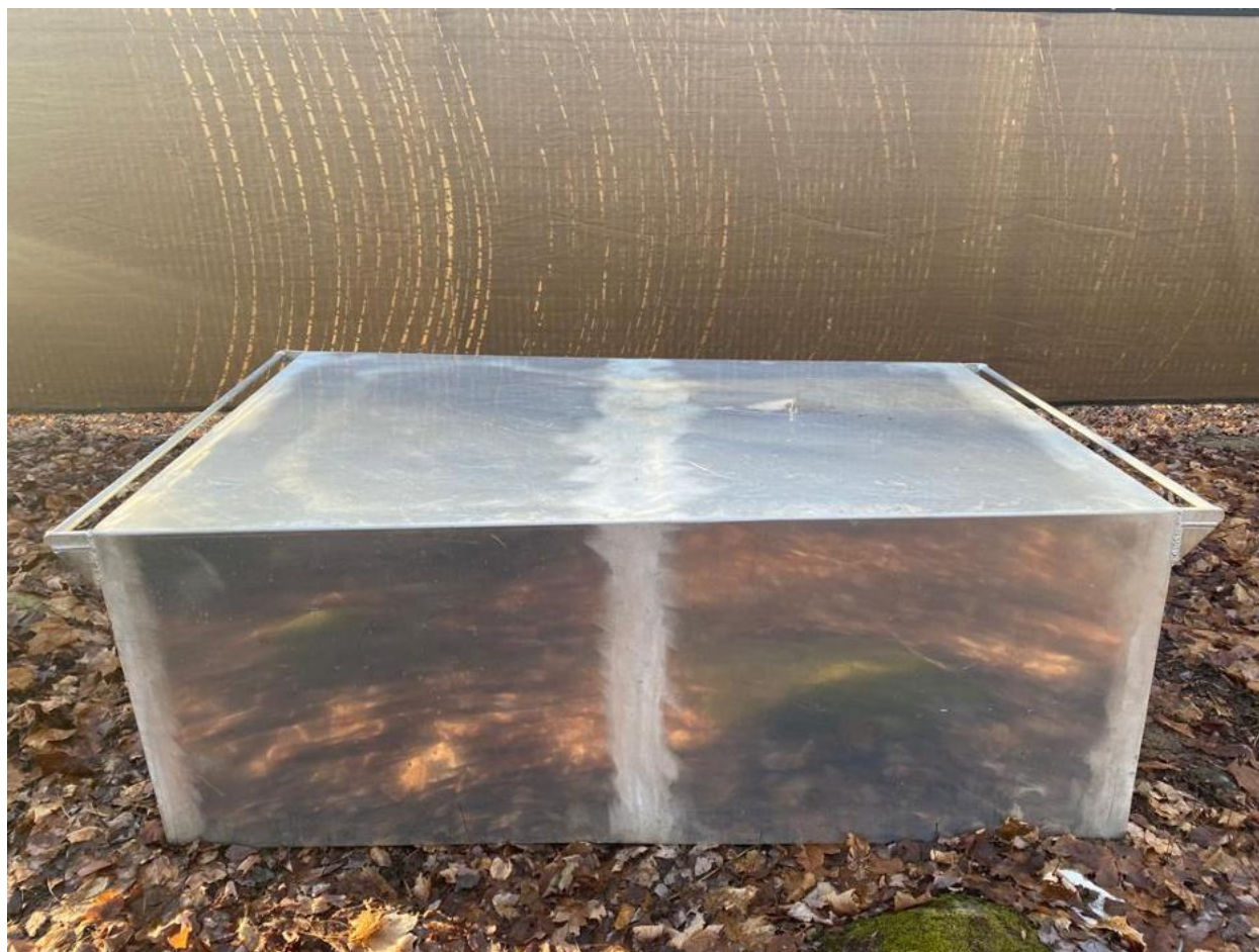
Figure 3-2 An aluminium hood (190 cm × 120 cm × 70 cm) placed over human remains for VOC accumulation at the REST[ES] facility.
