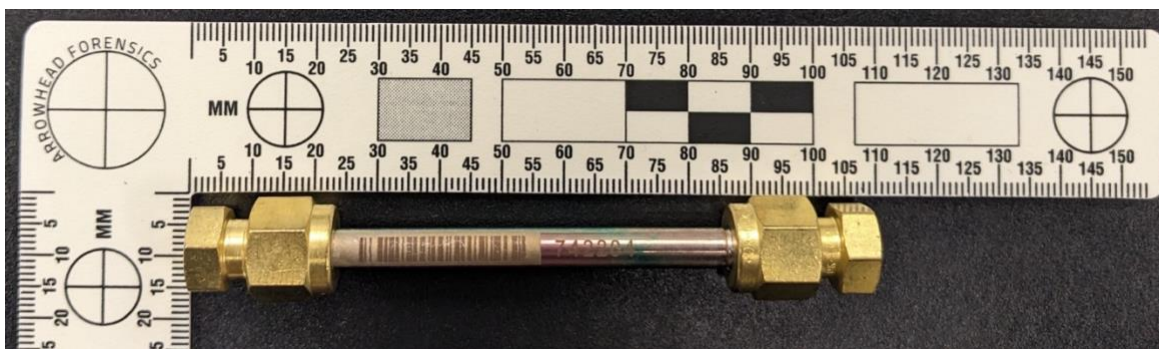
Figure 1-4 Stainless-steel dual sorbent tube with brass caps.
