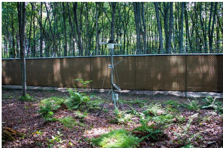
Figure 3-1 Hobo Weather Station (Onset Computer Corporation, Bourne, MA, USA) at the REST[ES] facility used to record measurements of ambient temperature ( ^{\circ}\text{C} ), rainfall (mm), relative humidity (%), wind direction ( \emptyset ), wind speed (m/s) and solar radiation ( \text{W}/\text{m}^2 ) every 15 min.
