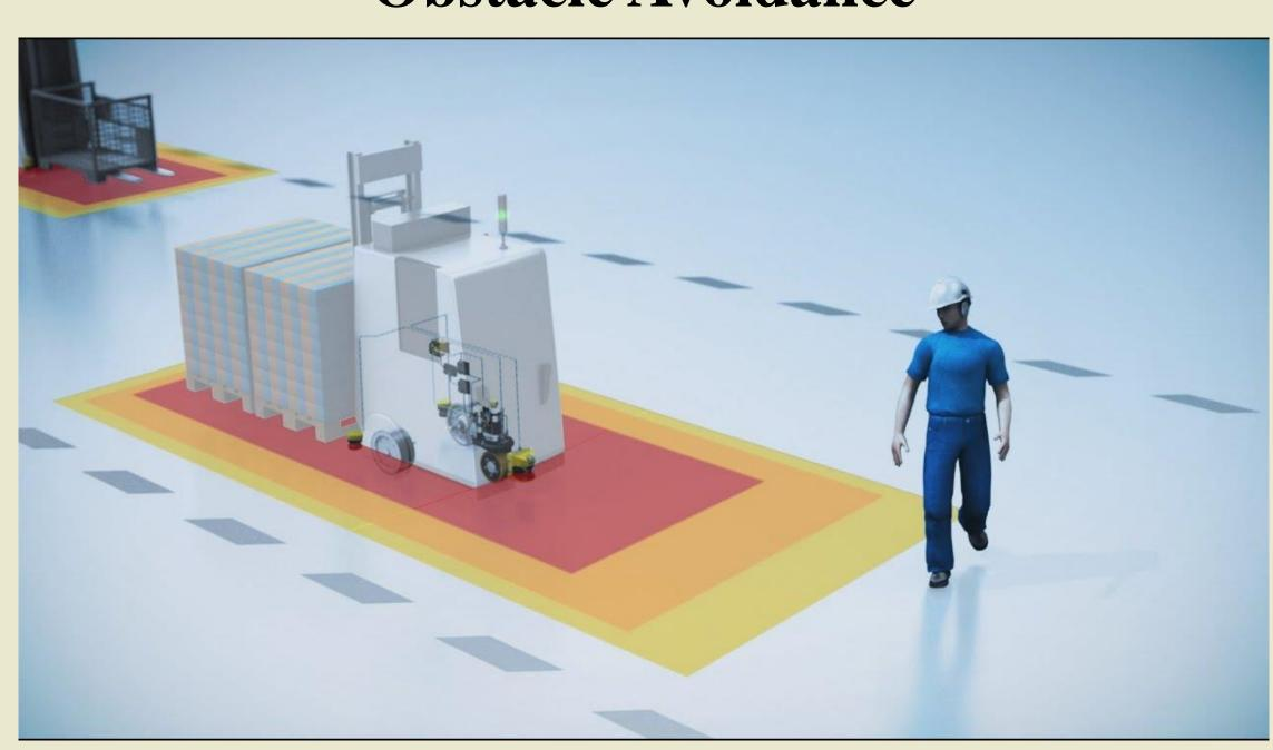
Obstacle avoidance is another problem for SGV. It must consider changes in environment to avoid unforeseen obstacles such as human and robot. Since static and dynamic obstacles can populate the navigation environment, the selection of an appropriate obstacle avoidance function is essential in motion planning.
