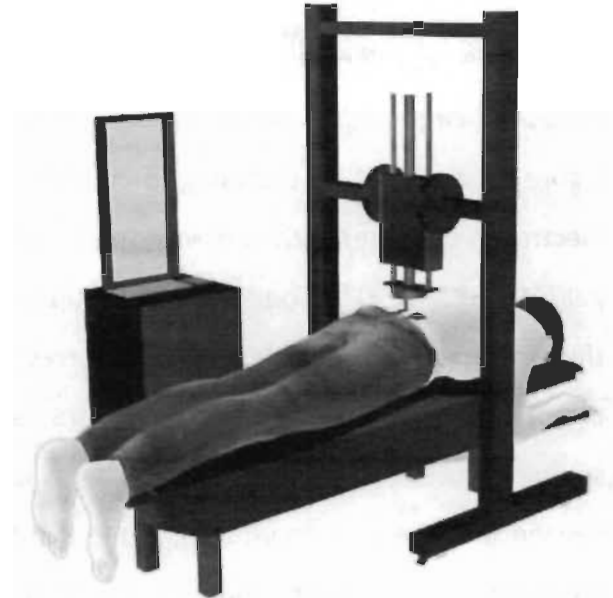
Figure 3.1. Representation of (a) the two large sEMG arrays of 64 electrodes used to record the neuromuscular response and (b) the experimental setup including the apparatus using a servo-controlled linear actuator motor. Each large sEMG array was located approximately at 2 cm from the L3 spinous process. sEMG: surface electromyography.
