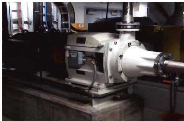
Figure 3.5 Raffineur conique Valmet RF-0
