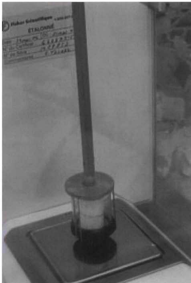
Figure 3-8 Sample holder with his stem mounted for the mercury intrusion test
