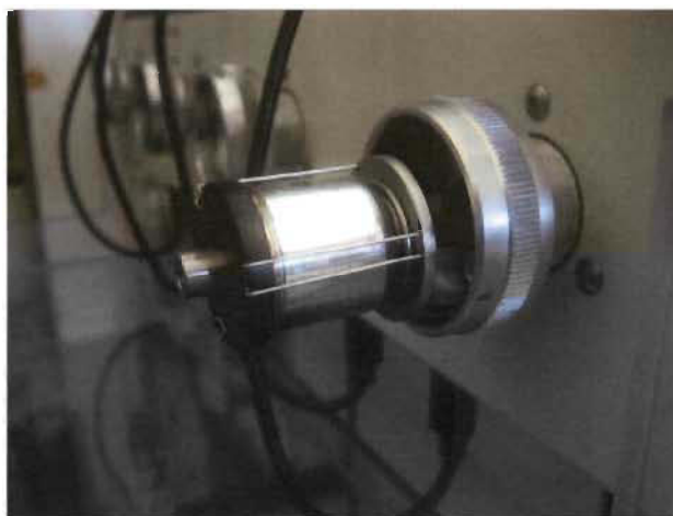
Figure 6-2 Bulb mounted for low pressure testing and fill with mercury
