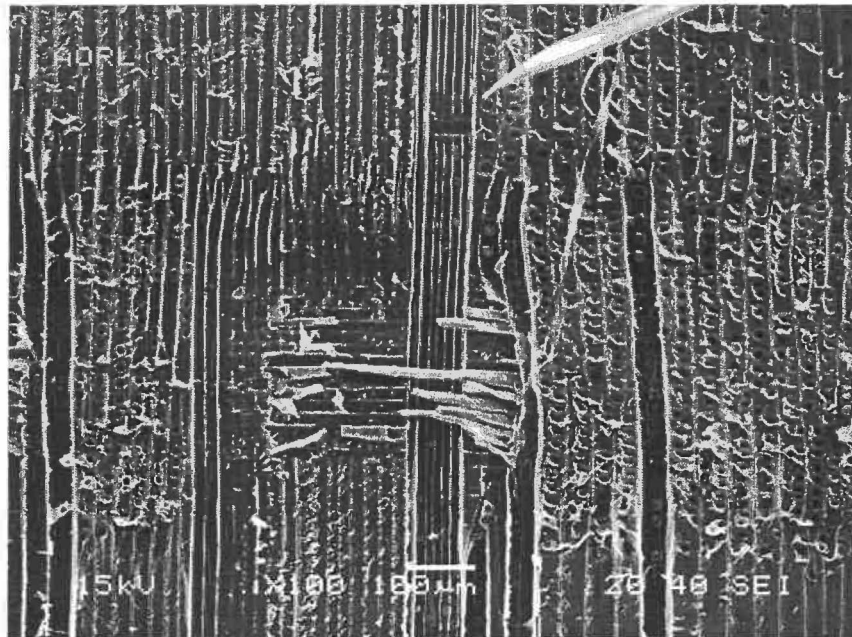
Figure 7.17 Radial fracture surface of uncompressed sample. Most fibers are separated in inter-cell mode and remained intact.
