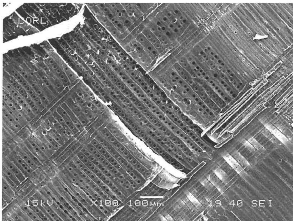
Figure 7.26 Radial fracture surface of uncompressed sulfonated sample. Fibers are separated in an inter-cell mode and remained intact.
