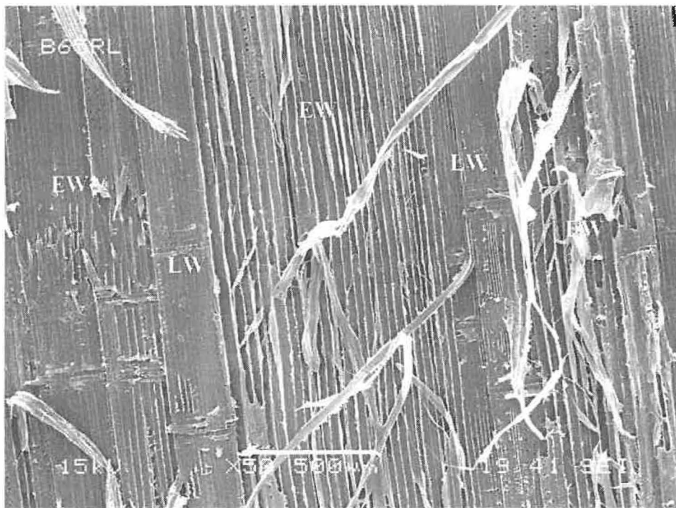
Figure 7.47 Radial fracture surface of sample compressed to 65% at 120°C. Most fibers are separated either in inter-cell and trans-wall mode.
