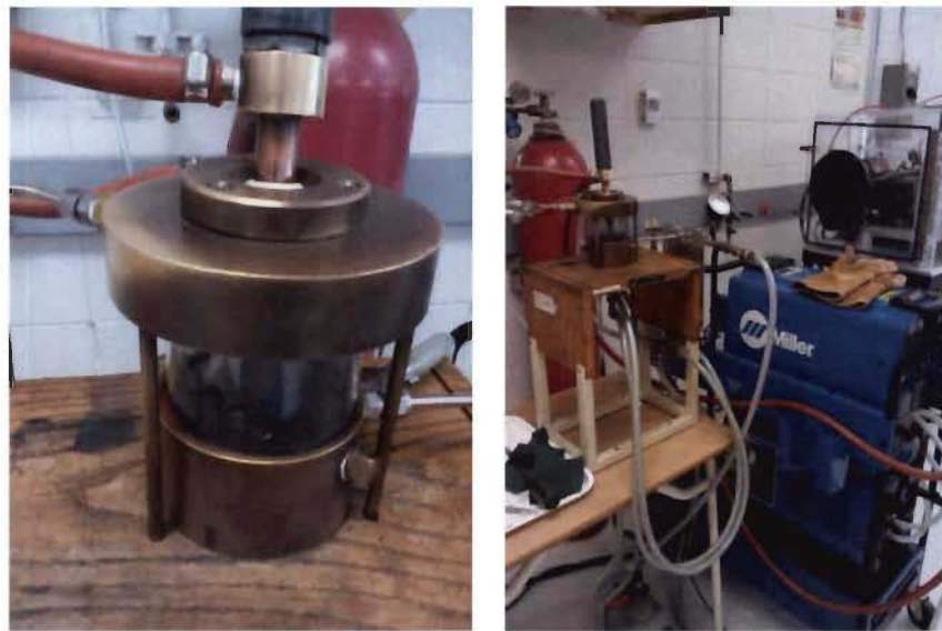
Figure 3.6- Arc melter (Centorr Associates Inc, USA).
