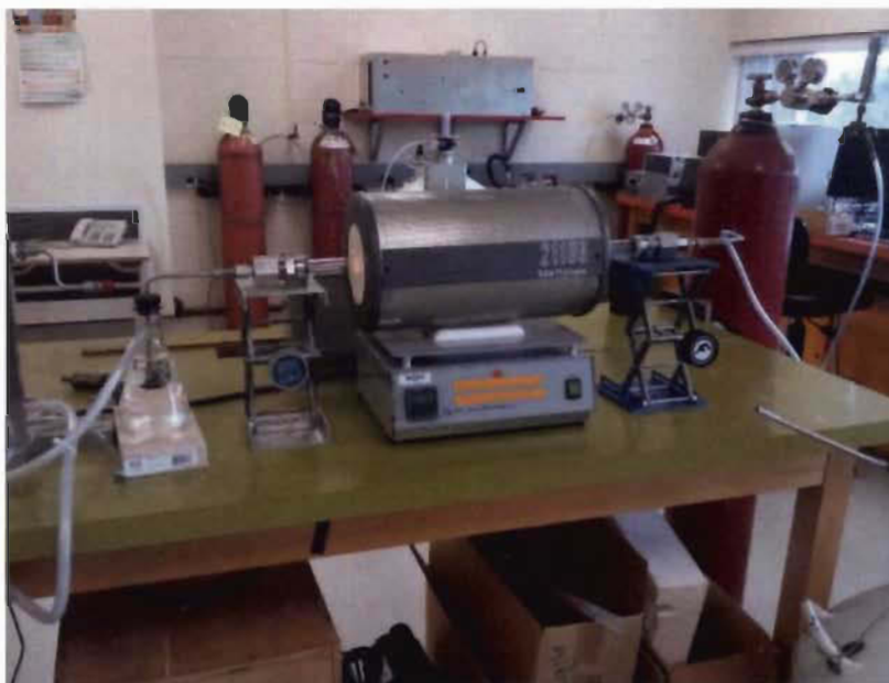
Figure 3.8- Heat treatment set-up with Tube furnace (Barnstead thermolyne).
