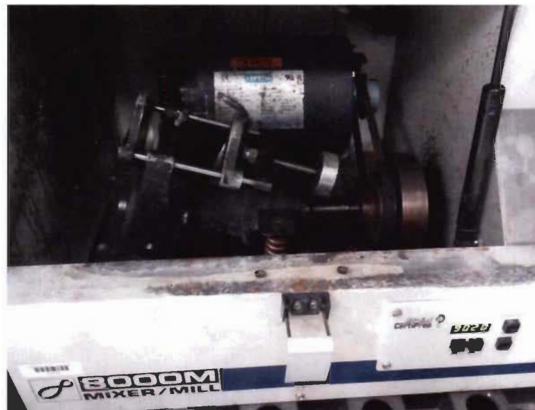
Figure 3.7- Ball miller Spex 8000M.
